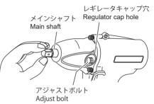
Set the torque by rotating the adjust bolt with pin. Positioning the main shaft front, by turning anti-clockwise, torque becomes higher and by clockwise, lower.
